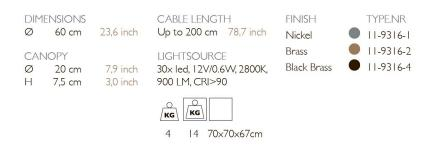
STANDARD The fixture is supplied with a black canopy with cover plate in matching colour of the fixture.
